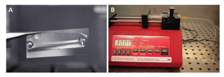
Figure 1. A) PDMS MFD for HUVEC cells culture under flow conditions. B) MFD connected to a syringe pump.
