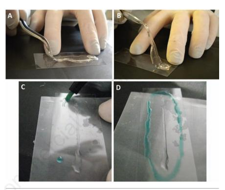
Figure 2. A-B) PDMS peeled from the glass. C-D) the area with cells attached to the glass, is outlined with an hydrophobic barrier pen (in green) to allow the immunostaining.
