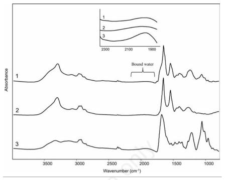
Figure 5. FTIR absorption spectra of cultured lymphocytes (1), albumin (2) and calf thymus DNA (3) after the fixative treatment with a solution of methanol:glacial acetic acid 2:1 followed by evaporation. The spectra are shown after correction of the Mie scattering and smoothing. A magnification of the spectral range between 2300 and 1800 cm<sup>-1</sup> due to bound water is also reported.
