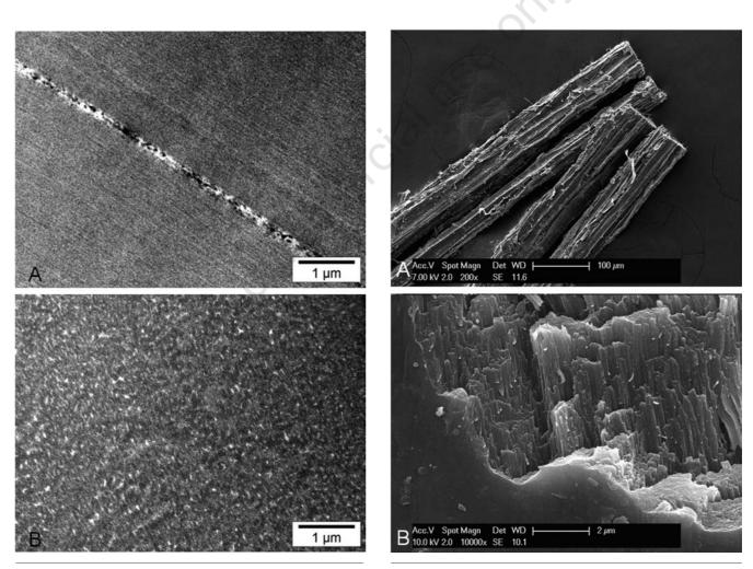
Figure 3. A) TEM micrograph of two adjoining fibres sectioned longitudinally; an ill-defined inner substructure, consisting of parallel microfibrillar material, is visible. B) TEM micrograph of a transected byssus fibre; the fibre appears to be a random mixing of two components of different electron-density. 14,000× magnification.
